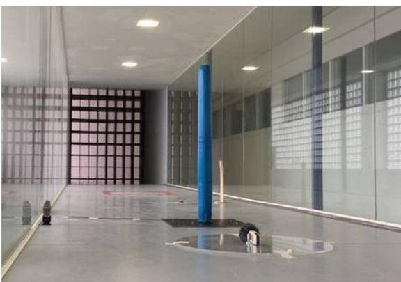
Figure 8. Testing device in the wind tunnel Acla16 in the CIDA (IDR/UPM). 1m height model, max. mast diam. 95mm and supported by a solid, circular section, 10cm diam., pultruded carbon fiber rod (February, 2018).
